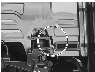
Position the mount and tighten the screw firmly so it does not come loose or damage the vehicle due to truck vibration.
