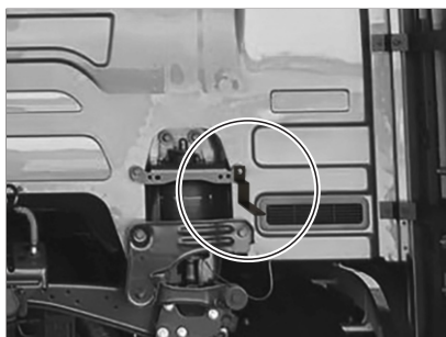
Position the mount and tighten the screw firmly so it does not come loose or damage the vehicle due to truck vibration.
