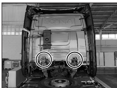
Area where the mount must be installed, passenger side.
